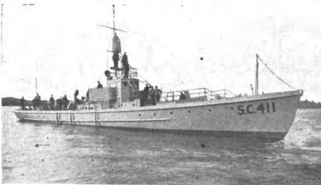
One of the 110 Footers Adopted by Uncle Sam When the armistice was signed, 406 of these boats had been commissioned. They were powered with three 250 h. p. Reversible gas engines manufactured by the Standard Motor Construction Company
