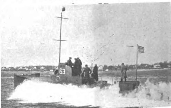
Type of Sub-chaser Used by Russian Government These were built by the Greenport Basin & Construction Co., at Greenport, Long Island, and are 60 ft. long, 9 1/2 ft. of beam and with two 8-cylinder Duesenberg engines made a speed of 30 knots
